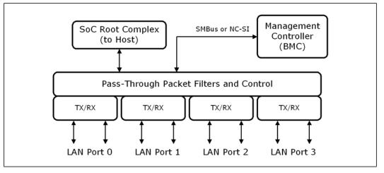
When an Ethernet packet reaches the GbE controller at the LAN Port, it is examined and compared to a number of configurable filters. These filters are configurable by the BMC and include, but not limited to, filtering on:
