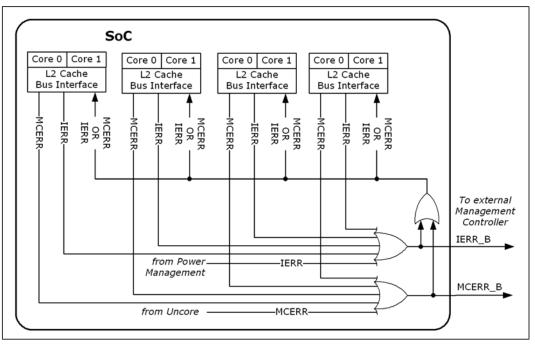
The IERR signal signifies a catastrophic internal error, a condition which requires immediate attention or possibly shutdown. When this error occurs, the processor core may not be able to execute reliably through the INT18 handler. The following are some possible cases of such catastrophic errors:
