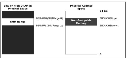
SMI handlers running on a CPU core execute out of SMM memory. To protect this memory from non-CPU core access, the **SMM Range** (BSMMRRL-BSMMRRH) is programmed anywhere in low or high DRAM space (1 MB aligned). This range only allows accesses from the CPU cores.
