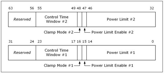
The units for the Power Limit and Control Time Window are determined as per the Package Power SKU Unit settings described in Section 17.9.2, "Package Power SKU Unit Read (Index = 30)" on page 418, while the valid range for power limit values are determined by the Package Power SKU settings described in Section 17.9.2, "Package Power SKU Unit Read (Index = 30)" on page 418 and Section 17.9.3, "Package Power SKU Read (Index = 28 and 29)" on page 419.
