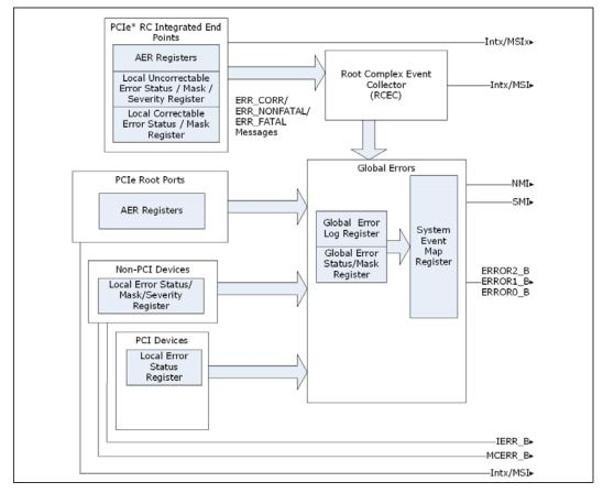
The SoC detects errors from the PCIe\* links and the SoC internal device errors. The errors are first logged and mapped to an error severity, and then mapped to a system event(s) for error reporting.
