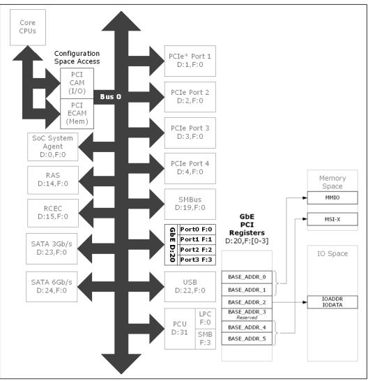
For details of the MMIO and MSI-X registers located in memory space and for the IOADDR and IODATA registers located in IO space, see the Intel<sup>®</sup> Atom<sup>™</sup> Processor C2000 Product Family Integrated GbE Controller Programmer's Reference Manual (PRM).
