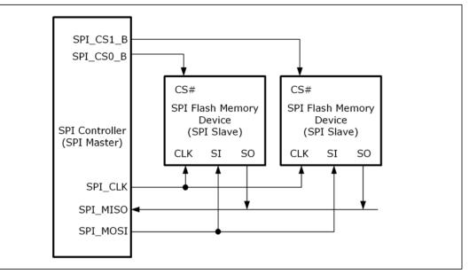
The SoC can boot the system BIOS and the system firmware through the Low Pin-Count (LPC) bus or through the SPI. The SoC detects from the hard straps which of these two BIOS/firmware boot sources to use. This is described further in Section 16.2, "Pin-Based (Hard) Straps" on page 357.
