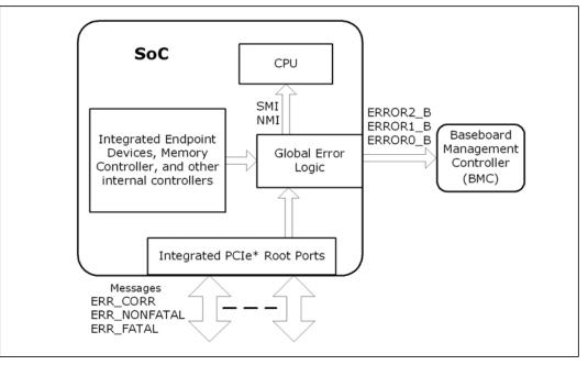
$\ensuremath{\mathsf{PCI}}\xspace$  error messages are received from downstream devices. The SoC logs these errors and other internal errors.
