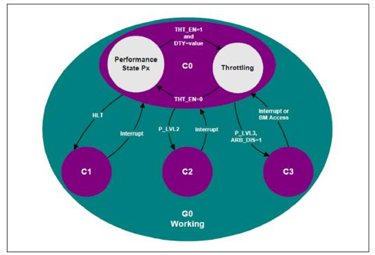
Concerning the SoC CMP Module and its interface to the System Agent, the SoC has three types of C-States:
